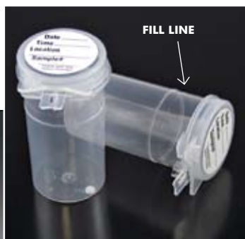
120mL flip-top container with 100mg sodium thiosulfate tablet
