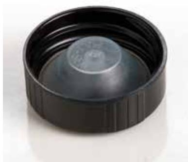
Phenolic caps are known for providing the widest range of chemical compatibility and for being the most temperature tolerant of plastic closures. The PE cone liner forms an exceptionally tight seal and provides a good chemical barrier.
