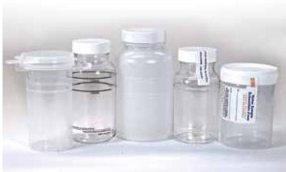
These sterile containers are used in testing for the presence of coliform, a microbiological contaminant in drinking water. QEC offers a variety of feature-rich sampling bottles, manufactured to the highest standards of precision and reliability.
