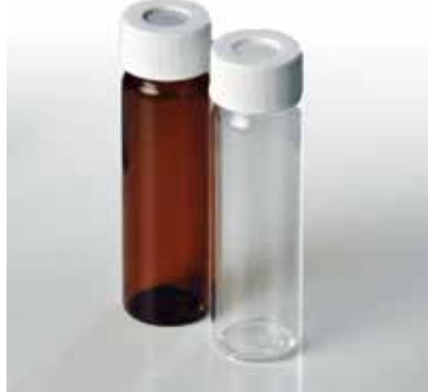
40mL EPA VOA vials in clear 33 expansion or amber 51 expansion borosilicate glass, assembled with solid PTFE septa disc inserted in polypropylene cap.
