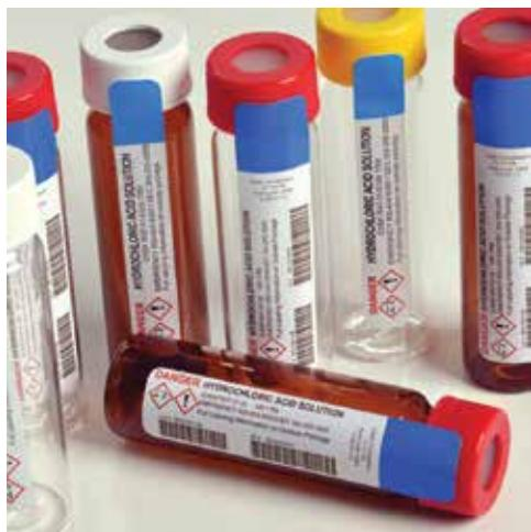
40mL VOA vials preserved with 1:1 Hydrochloric Acid (HCl) solution, for use in preserving samples containing volatile organic compounds.
