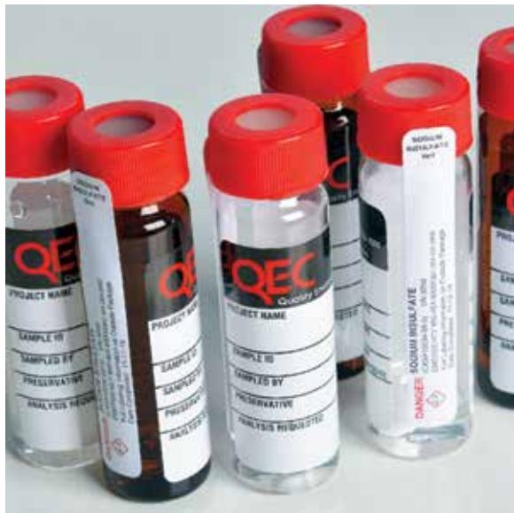
QEC's Method 5035 preserved vials are 40mL Level 3 VOA vials (pre-cleaned to EPA standards, with Certificate of Analysis), with open-top caps and low-bleed 0.125" PTFE/silicone septa. Prepared with label and tamper-evident seal.
