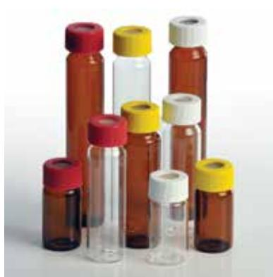
VOA VIALS are most often used for volatile organic compound analysis. Available in clear 33 expansion and amber 51 expansion borosilicate glass. Open top vials come assembled with polypropylene caps with low-bleed 0.125" PTFE/silicone septa inserted (.135" septa for E-series vials). Sizes are 20mL, 40mL, and 60mL.
