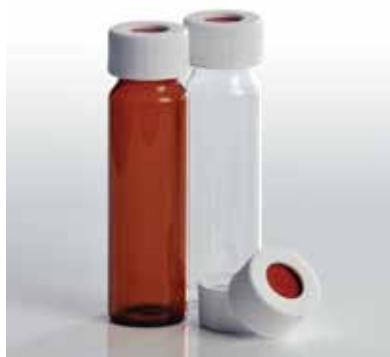
40mL EPA VOA vials in clear 33 expansion or amber 51 expansion borosilicate glass, assembled with 0.060" PTFE/chlorobutyl septa disc inserted in polypropylene cap.
