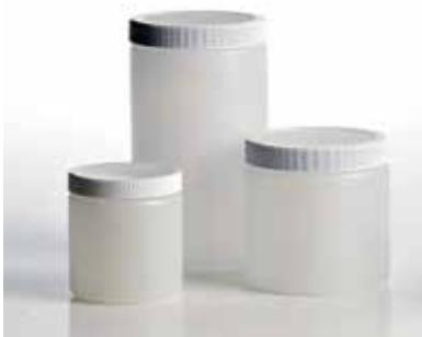
QEC HDPE Straight Sided containers feature an extra wide opening and jar style to allow for easy insertion and recovery of contents. Polypropylene caps with foamed polyethylene liners have excellent sealing, with good chemical resistance to acids, alcohols, alkalis, aqueous products, oils and solvents. Prepared containers come assembled with cap and liner.
