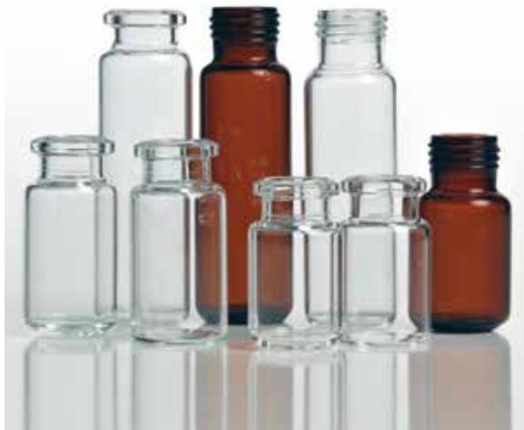
QEC headspace vials are available in 6, 10 and 20 mL sizes. It is recommended that you use a large enough vial to ensure adequate headspace phase ratio.
