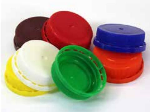
Locking caps fit QEC HDPE dairy jugs and juice bottles that have a ratcheted 38-400 finish. Caps are sturdy polypropylene with ribbed sides and an interior sealing ring, as well as the ratcheted locking ring.
